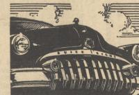
FOUR-WAY FOREFRONT This rugged front end (1) sets the style note, (2) saves on repair costs—vertical bars are Individually replaceable, (3) avoids "locking horns," (4) makes parking and garaging easier.
