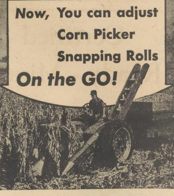
It's new! It's exclusive! It's another great International Harvester development! Now, you can adjust McCormick corn picker snapping rolls on the go - from the tractor seat! Pushing or pulling a handy lever gives you eight different snapping roll spacings.
