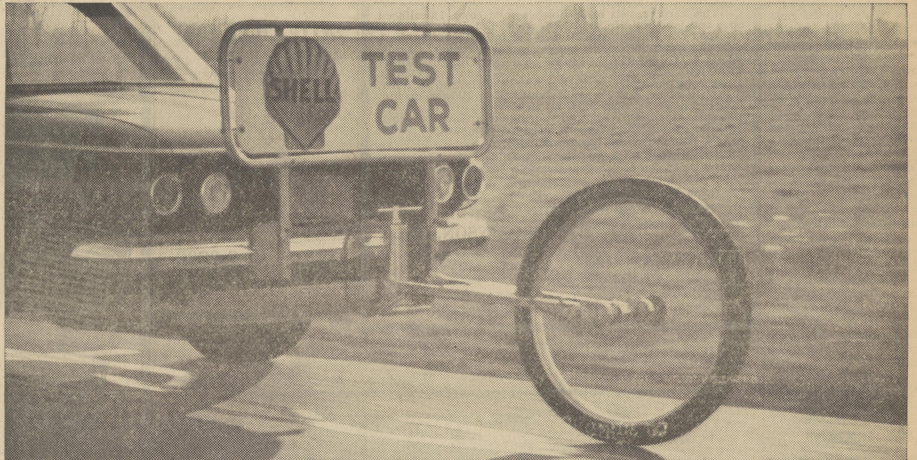
Shell test drivers add a "fifth wheel" to their cars for precise distance measurement during mileage tests. It helps them record performance to a decimal point.
