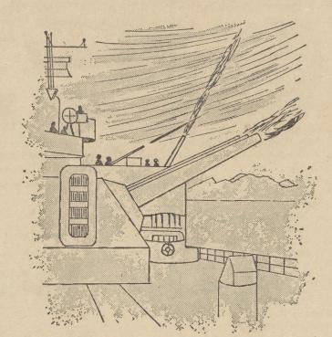
The USS HELENA has been fitted for "Regulas" guided missiles, although it is not classified as a guided missile cruiser. She displaces 13,600 tons std. and 17,200 tons fully loaded. Some of her big guns include 9-8 inchers, 55 cal.; 12-5 inchers, 38 cal.; and 52-40MM. Like most cruisers she carries a helicopter.
