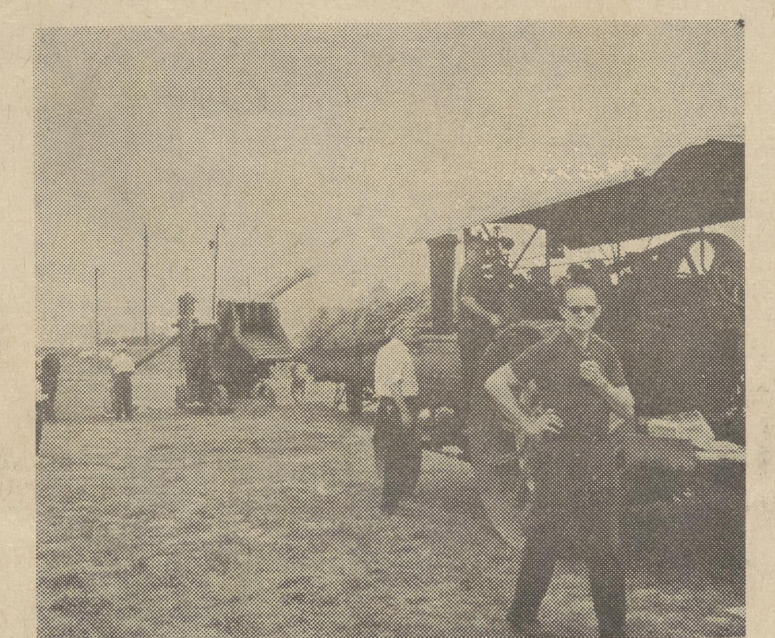
STEAM ENGINE used to run wheat thresher in the binning process of wheat threshing.
