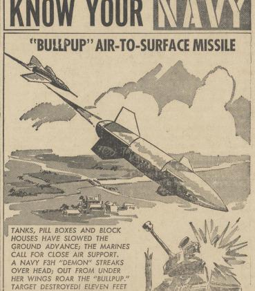
LONG AND WEIGHING ONLY 540 POUNDS, "BULLPUP" IS AN AIR-TO-SURFACE MISSILE DESIGNED FOR USE AGAINST TOUGH GROUND TARGETS. INEXPENS AND RELA-
