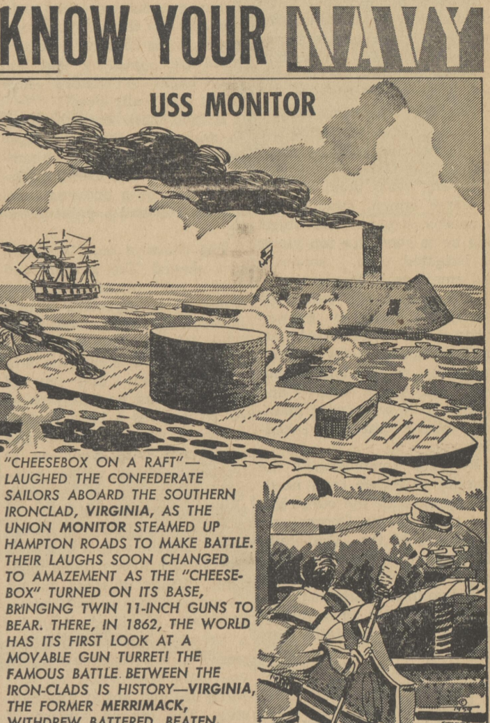
"CHEESEBOX ON A RAFT" - LAUGHED THE CONFEDERATE SAILORS ABOARD THE SOUTHERN IRONCLAD, VIRGINIA, AS THE UNION MONITOR STEAMED UP HAMPTON ROADS TO MAKE BATTLE. THEIR LAUGHS SOON CHANGED TO AMAZEMENT AS THE "CHEESEBOX" TURNED ON ITS BASE, BRINGING TWIN 11-INCH GUNS TO BEAR. THERE, IN 1862, THE WORLD HAS ITS FIRST LOOK AT A MOVABLE GUN TURRET IN THE FAMOUS BATTLE BETWEEN THE IRON-CLADS IS HISTORY-VIRGINIA, THE FORMER MERRIMACK, WITHDREW BATTERED, BEATEN.
