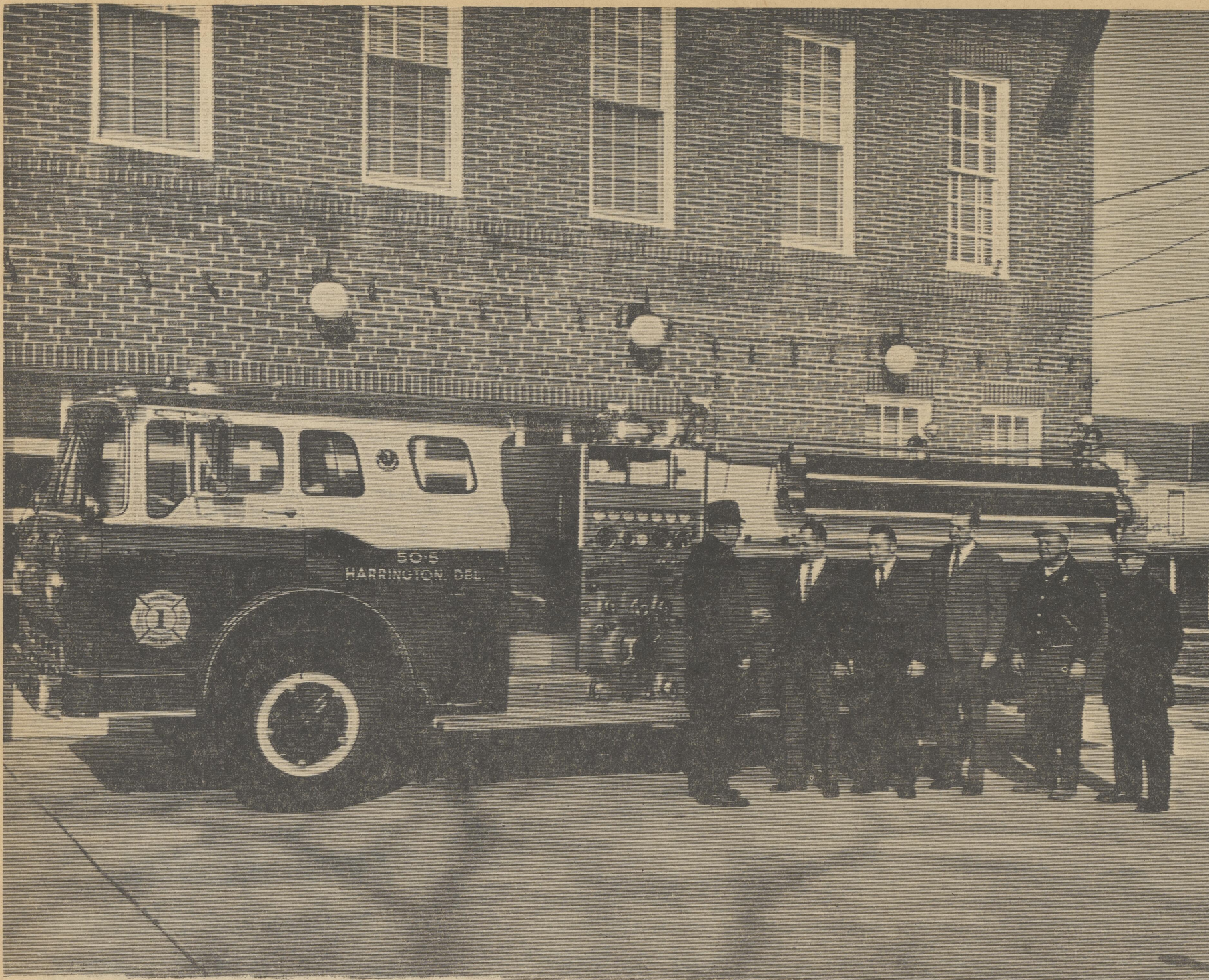
NEW 1000 GPM TRIPLE COMBINATION PUMPER recently delivered to the Harrington Vol. Fire Dept. on 12/30/69. The chassis is a C-1000 Ford, OLD-10 Hale Pump, and the body was built by Hahn Motors, Inc., Hamburg, Pa. Pictured inside the pumper from left to right are: Joe Webb (owner of Webb Ford's Mercury Inc., Milford, Del.) presenting the keys and a check in the amount of $200 donation to the truck Purchasing Committee: Harold E. Fry, Robert A. Wilson, Melvin R. Wyatt, Ira Hoffman, and William H. Cotten.
