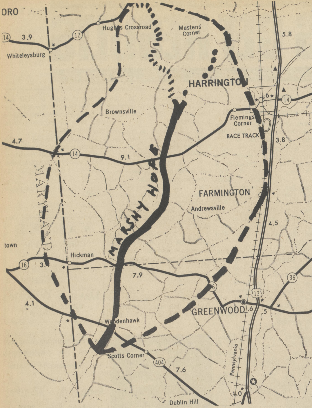
MARSHY HOPE TAX DITCH COMPLETED —The waterway, indicated by the heavy line, drains about 56,000 acres. Construction will begin next month on the Horsepen Arm Tax Ditch, indicated by the barred line extending from Marshy Hope. The Black Arm Tax Ditch, indicated by the dotted line from the Marshy Hope Ditch, will begin construction later this year.
