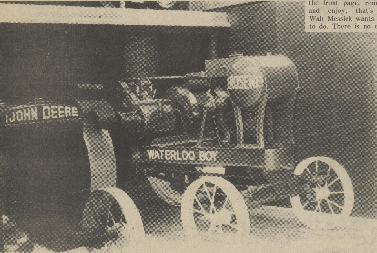
THE WATERLOO BOY, a kerosene fueled early John Deere tractor, is the first antique farm item Walter Messick acquired. In the 28 years since that
