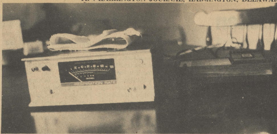
The apnea monitor, [left front] the harness of the monitor and portable intercom work together to detect breathing irregularities.
