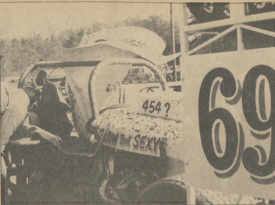
Richard Johnson's #69 after the crash on the first turn. Note the right side which is pushed in on the driver. The top of Johnson's car was cut off to enable him to be pulled out of the car.
