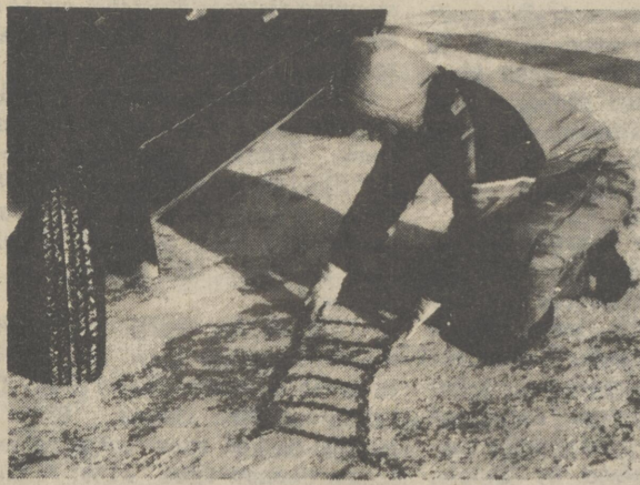
STEP NO. 1 Spread the chains on the ground to remove twists or tangles. Make sure the cross chain hooks are facing up.
