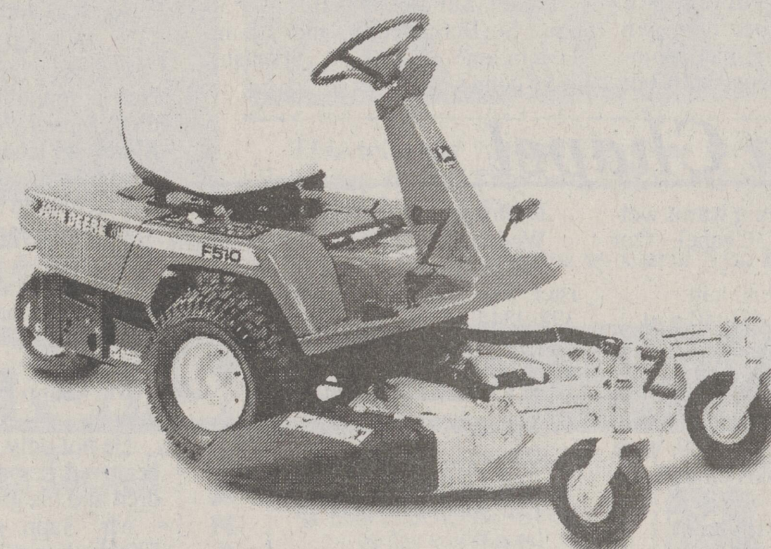
The F510 with 38-inch cutting deck and a 14-hp overhead-valve engine.
