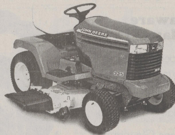
The 325 with 48-inch cutting deck and a 17-hp overhead-valve engine.
