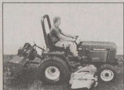
955 Compact Utility Tractor • 33-hp diesel engine • Hydrostatic transmission
